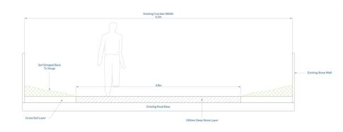
Figure 8-5: Typical Cross-Section (Section W)
