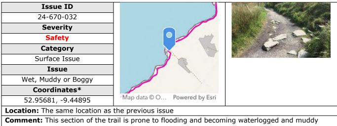
**Comment:** This section of the trail is prone to flooding and becoming waterlogged and muddy making the unofficial trail close to the cliff edge a more attractive route. Trail upgrade needed to prevent flooding and signage needed to warn walkers not to climb the barrier.
