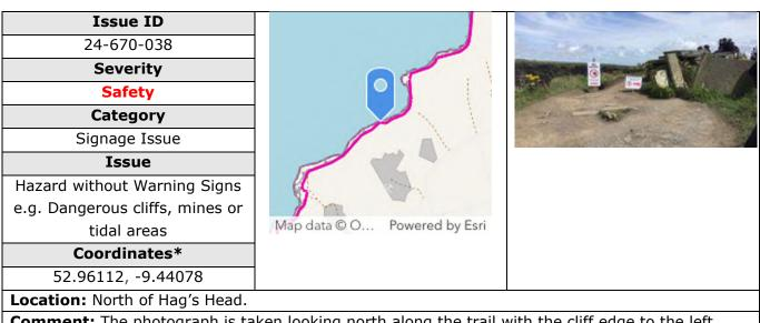
**Comment:** The photograph is taken looking north along the trail with the cliff edge to the left. Here the official trail to the right is through a 'stile' made of two flagstones placed in an upturned V. This presents a visual barrier to the trail user and presents an unnecessary obstacle. This stile should be removed. The warning signage should be accompanied by a fence preventing walkers from using the very dangerous unofficial trail to the left.
