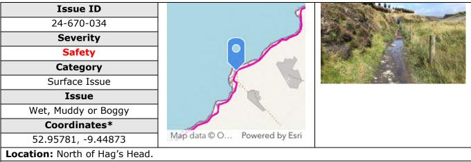
**Comment:** Looking north along the trail the photograph shows the majority of trail users walking the unofficial path at the top of the high earthen barrier. The official trail on the right is waterlogged and very narrow and there are no warning signs directing walkers not to climb up to the unofficial path. This trail surface here needs to be upgraded and the trail widened ti allow for the large number of trail users.
