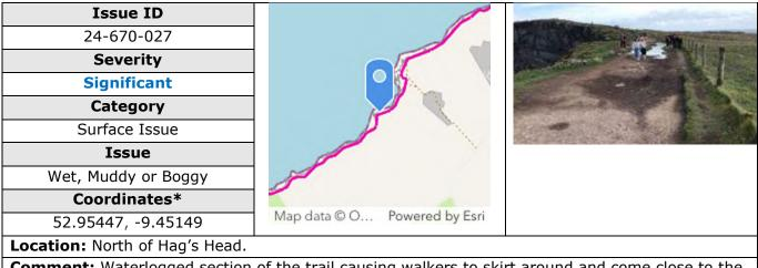
**Comment:** Waterlogged section of the trail causing walkers to skirt around and come close to the cliff edge. Trail upgrade needed and/or fencing and warning signage.
