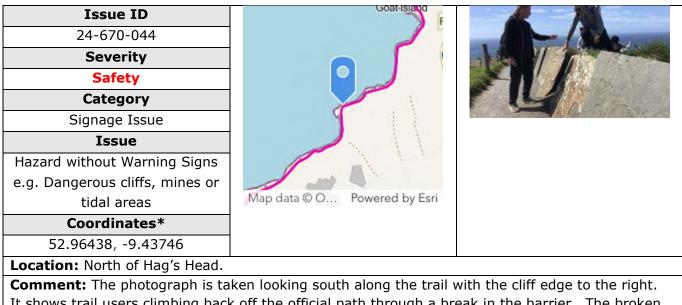
It shows trail users climbing back off the official path through a break in the barrier. The broken section of barrier should be repaired and signage erected reminding walkers to stay on the official path and not to cross the barrier.
