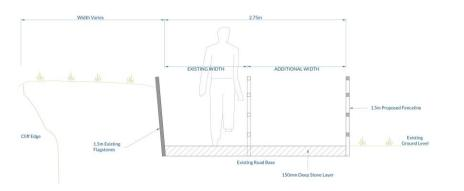
Figure 8-6: Typical Cross-Section (Sections X and Y)
